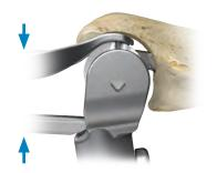
Align Bearing tabs with slots in Humeral Implant
